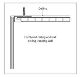
This method of installation uses a edging strip 2-part profile. Connect part one (backing strip) of the edging strip to the ceiling using a suitable silicone and fix with a screw through the long edge of the profile. It is recommended to use a larger amount of silicone against the connecting edge of the sheet to ensure a watertight installation. Place the ceiling plank into the correct position and clip in the part two facing strip into place.
