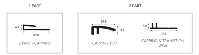
Capping profiles are used to create a watertight seal between the sheet and the ceiling/flooring.
